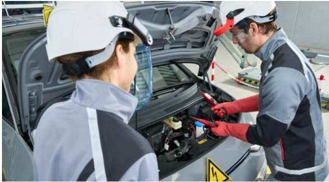
Testing the high DC voltage of a HV electric vehicle.
