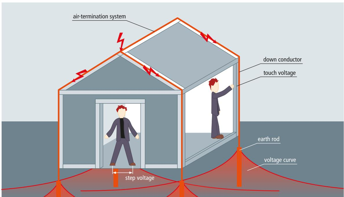
Figure 9.28.1 Risk due to touch and step voltage
