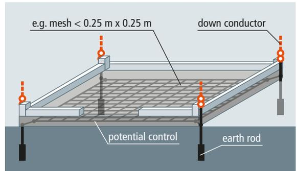
Figure 9.28.5 Potential control to reduce step voltage
