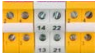
Floating remote signalling contact DRC MCM XT: break contact (21/22), make contact (13/14) DRC SCM XT: break contact (21/22)
