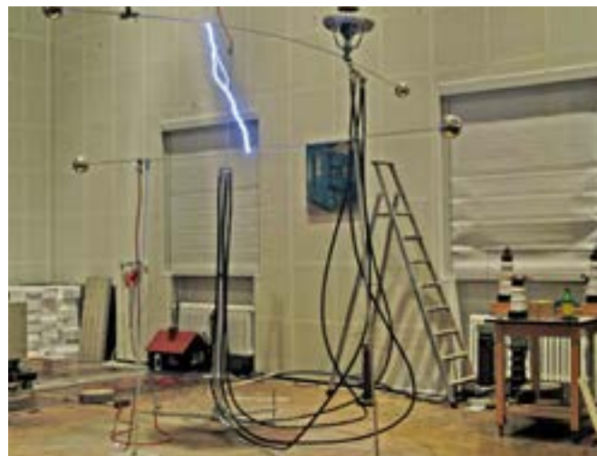
Figure 6: High voltage test according to IEC TS 62561-8 Edition 1.0 2018-01 of a HVI system with four HVI Conductors.
