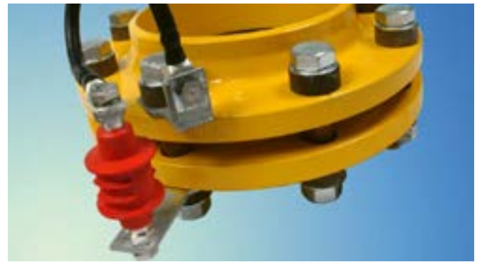
ATEX and IECEx-certified isolating spark gap with a low sparkover voltage for lightning equipotential bonding according to IEC 62305.
