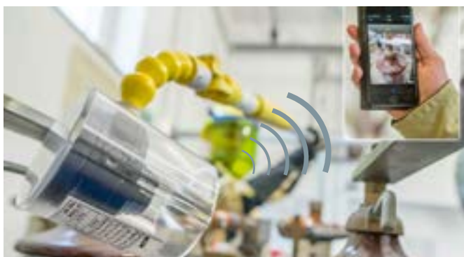
Live inspection of an insulator on its rear side.
