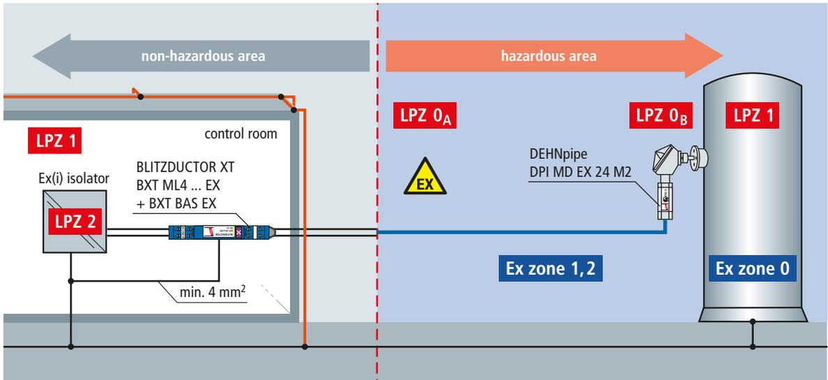
Figure 9.32.4 Surge protective devices in an intrinsically safe measuring circuit
