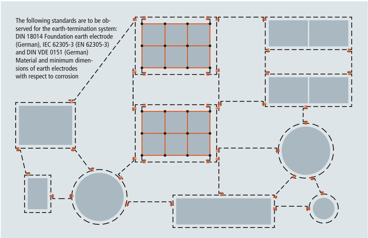
Figure 9.32.6 Example of an intermeshed earth-termination system
