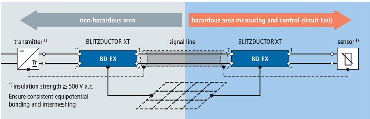
Figure 9.32.7 Example of the shield treatment of intrinsically safe cables
