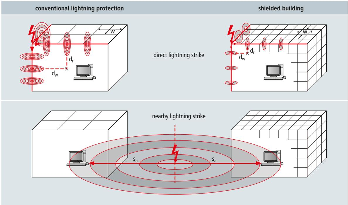
Figure 9.32.3 Shielding of structures by using natural components of the building
